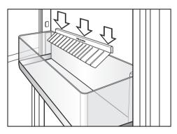
Attach the bottle holder centrally along the rear edge of the bottle shelf, as shown.
